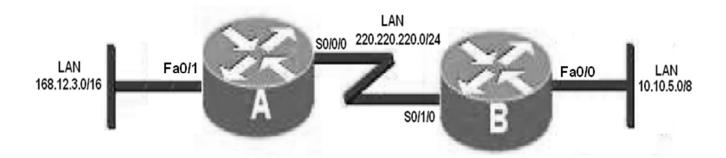
According to the previous information, which are the two commands that allow connectivity between 168.12.3.0 and 10.10.5.0 networks without recurrent search?
